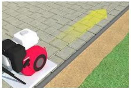
**8.** Spread more sand over the surface and sweep it into crevices between pavers. This step may need to be repeated over the next couple of weeks.
