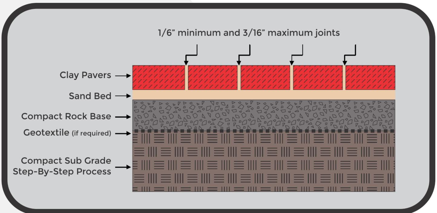
1. Excavate the area to be paved using a shovel or skid loader. The depth needed will depend on the intended use for the paved area. If the area will be used for foot traffic only, you will need a
